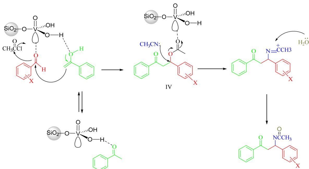
**Scheme 4.** The proposed mechanism for the formation of  $\beta$ -acetamido ketone catalyzed silica vanadic acid.
