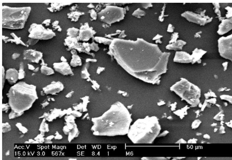
**Fig. 4.** The SEM image of RHDNPH.
