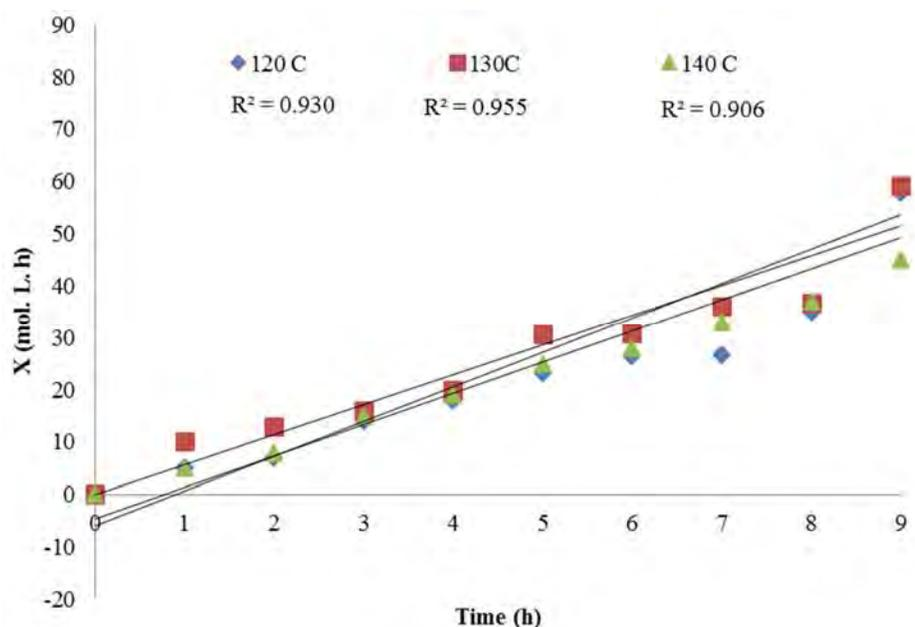
**Fig. 6.** The pseudo zero rate plots for the hydrolysis of cellulose over the surface of RHDNPH. The correlation coefficients were also shown.
