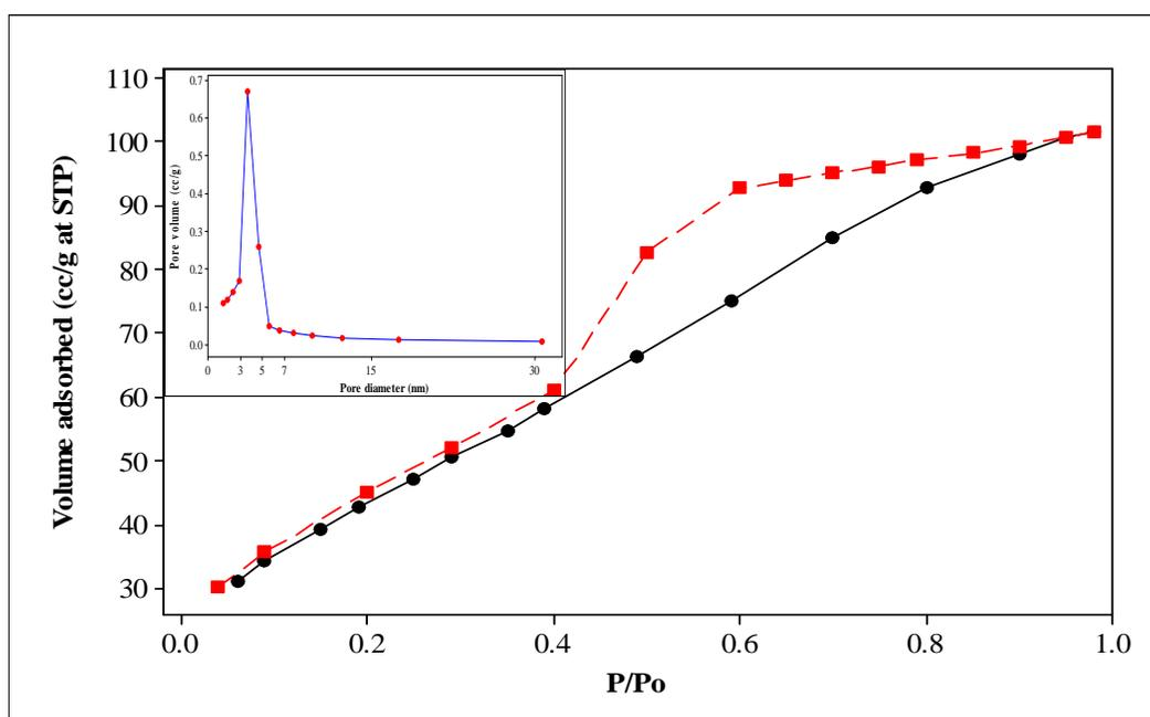
**Fig. 2.** The  $\text{N}_2$  adsorption/desorption isotherms of RHDNPH with the corresponding pore size distribution inset.
