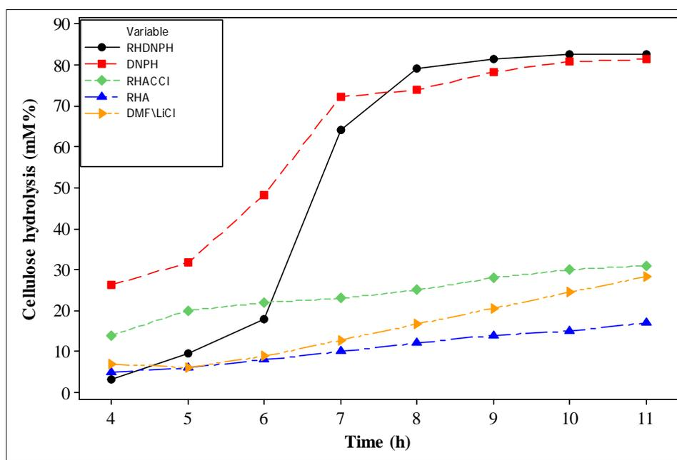
**Fig. 5.** The hydrolysis of cellulose to glucose over RHDNPH, RHA, RHACCl, DNP and DMF/LiCl without catalyst as a function of hydrolysis time.
