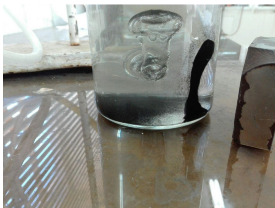
Fig. S4. Magnetic effect of MPCAC catalyst under the influence of magnet.
