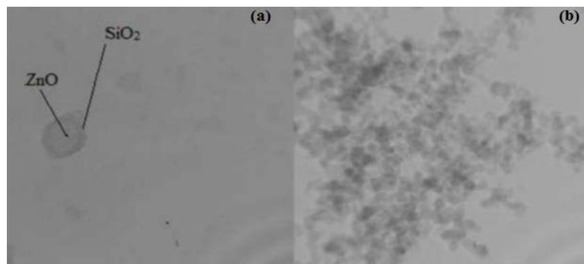
**Fig. 3.** TEM micrograph of the APTES modified ZnO@SiO<sub>2</sub> nanoparticles. (a) A higher magnification image, (b) Overview.
