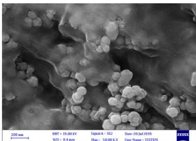
Fig. 4. FESEM image of GO-ZnO@SiO<sub>2</sub> hybrid.
