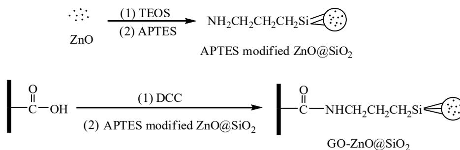
**Scheme 2.** The fabrication of GO–ZnO@SiO<sub>2</sub> hybrid.
