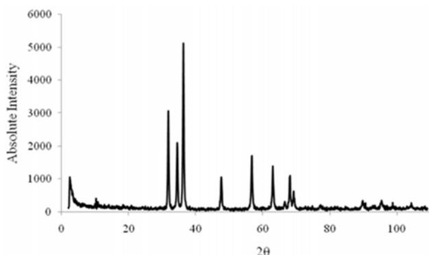
**Fig. 1.** XRD patterns of ZnO nanoparticles.
