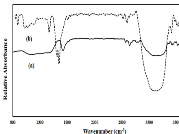
Fig. 5. FTIR spectra of (a) GO and GO-ZnO@SiO<sub>2</sub> hybrid.
