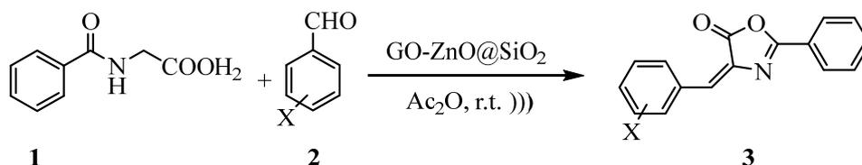
**Scheme 1.** The Erlenmeyer–Plöchl reaction for the synthesis of azlactones under ultrasonic irradiation.
