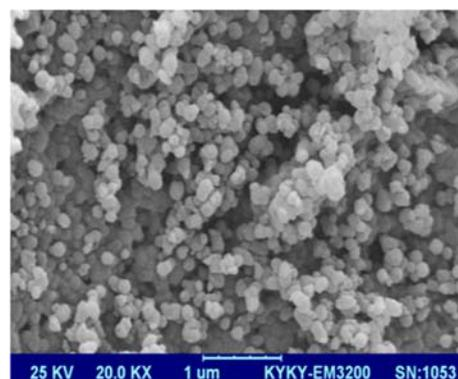
**Fig. 2.** SEM images of ZnO nanoparticles.
