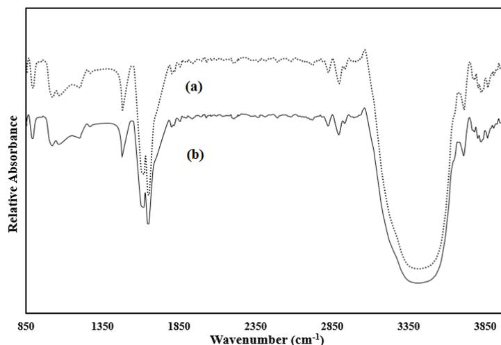
**Fig. 6.** FT-IR spectra of catalyst, before (a) and after (b) use.**Table 3.** Comparison of the reported methods for the condensation of benzaldehyde with hippuric acid in different conditions.
